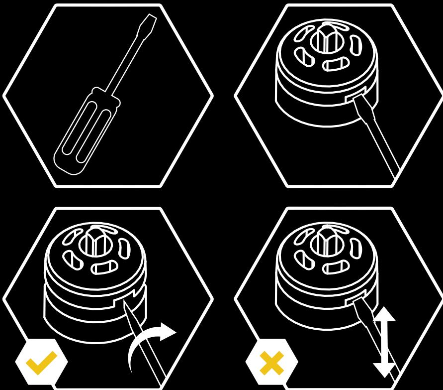
**EN.** When removing your valve cap for cleaning ensure that the screwdriver is twisted and NOT prised.
